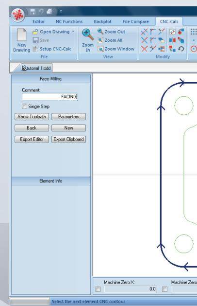
CIMCO CNC-Calc performs geometric calculations and toolpath creation in seconds. Supports 2D strategies for milling and turning
