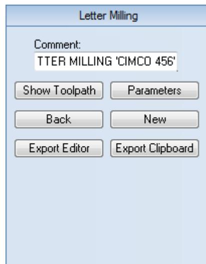
Next, click on the **Parameters** button. The TrueType Text Milling Parameters dialog appears. Check the **Mill Outline** option at the top and fill in the rest of the fields as shown below. Click **OK** when done.
