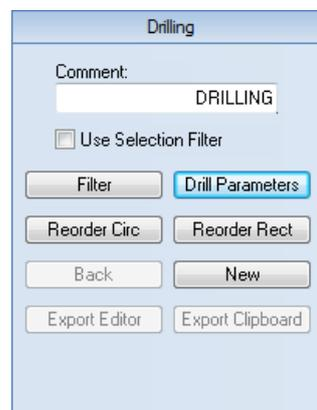
Click on the button **Drill Parameters** to open the parameter dialog window shown below. For this drilling operation, please enter the parameters shown.
